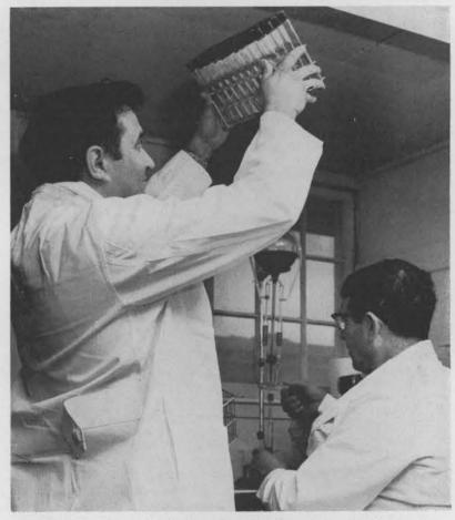
TEST TUBES are checked against light by Alexander Jack after 24 hour incubation period for visible signs of gas bubbles, indicating bacteria. Richard Sanchez fills tubes for additional tests.
